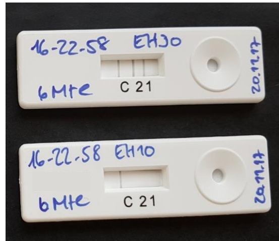
Image 1: The top test strip shows a positive result where the two bacterial strains were successfully detected. The bottom test strip shows negative results where there was no bacterial strain detected whatsoever.
