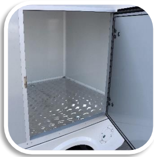
Cargo steel floor
