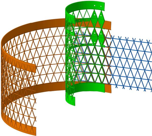
*Figure 4: Overlay of the different test samples to be fabricated in the CTP development: blue – flat panel for rib and node tests, green – 0.5m diameter cylinder of high complexity, orange – simplified full scale lattice cylinder. All samples feature identical cell geometries for tooling reuse.*
