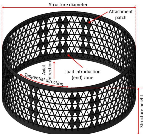
Figure 3: Lattice structures terminology.
