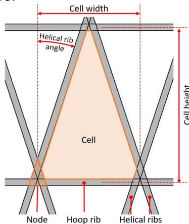
Figure 2: Lattice structures terminology.
