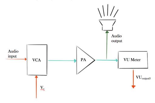
2.1.2 Audio Amplifier System Diagram - Automatic Volume Control
