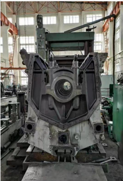
Boring the main bearing hole of the HXN3 engine block
