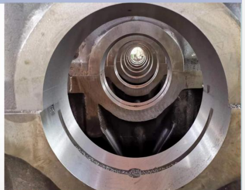
Boring the main bearing hole of the HXN3 engine block
