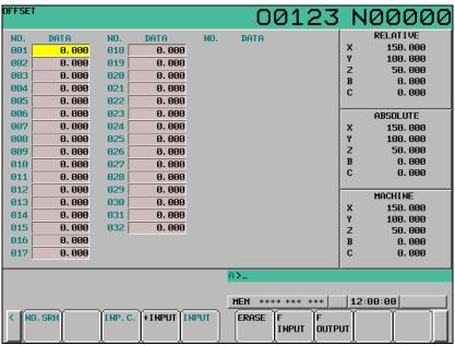
Fig. 1.1.1 (a) Tool compensation memory A (10.4-inch)
