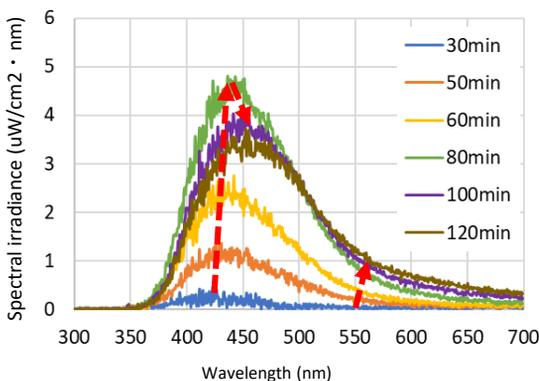
With oxidation, a long wavelength shift was observed in the peak position in the 400nm range, and an increase in intensity was observed in the long wavelength region of 550nm and above.
