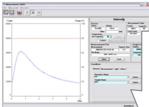
The amount of luminescence at all wavelengths is measured for each exposure time setting (0.1 sec, 1 sec, 10 sec). The degree of oxidation is determined by parameters such as the height, slope, time and total area of the luminescence peak.
