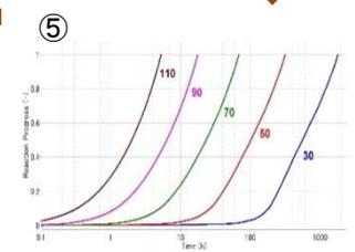
This suggests that lifespan can be predicted by means of CL measurement under multiple temperature-elevation measurements, without acceleration testing.
