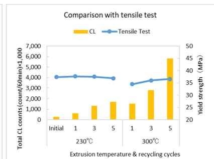
The higher the recycling cycle count, the higher the amount of luminescence shown; slight oxidation due to recycling could be detected. In the physical property tests (the flexure test and tensile test), hardly any difference was observed.
