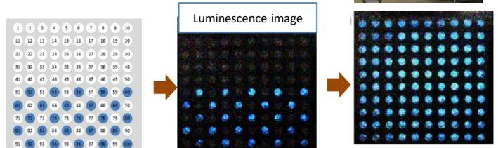
OIT measurement was carried out simultaneously on 100 samples. In the PP without the antioxidant, the OIT was shorter, and the OIT time course could be detected with good reproducibility, without being affected by adjacent samples.
