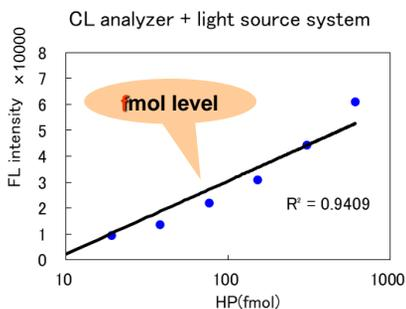
In contrast to the method using a general fluorescence spectrophotometer, this method enabled a calibration curve to be obtained to about 20fmol.
