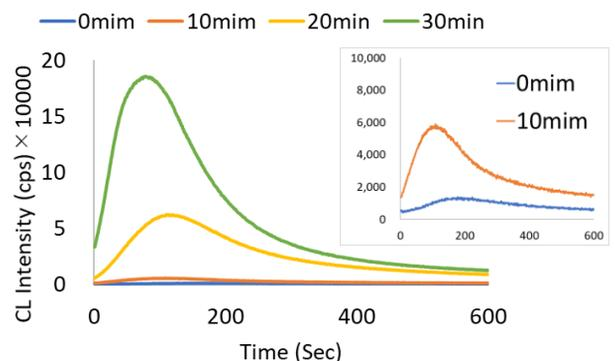
With the infrared absorption measurement method, a peak derived from the carbonyl group was visible in the sample after 30 minutes of heating (see graph on left), but with the CL method, an increase in luminescence was observed after 10 minutes of heating.
