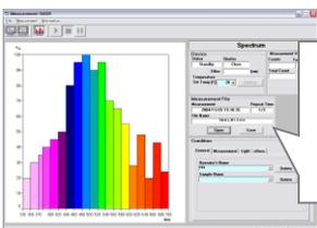
Spectrum measurement is performed while the spectral filter (high-pass filter) built into the device rotates automatically.
