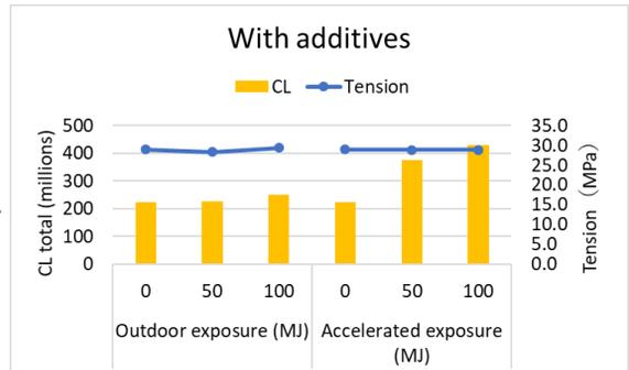
The "with additives" exposure-tested samples showed only a slight difference, but the acceleration-tested samples showed an increase in the amount of luminescence as they degraded, indicating a small difference in oxidative degradation at the very beginning.
