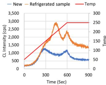
The amount of luminescence was higher in the sample refrigerated for 2 years than in the new sample, and multiple luminescent components were observed by means of temperature-elevation measurement.
