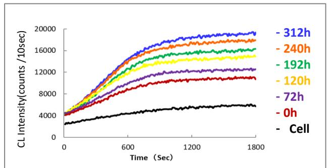
The longer the thermal oxidation time, the higher the amount of luminescence (see graph above); the integrated amount of luminescence at 1,800sec showed a high positive correlation with the thermal oxidation time (see graph on left).
