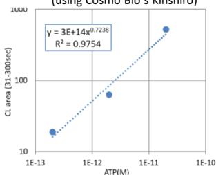
Luminescence up to about  $1 \times 10^{-13}$  M showed good linearity, with a correlation coefficient of 0.97.
