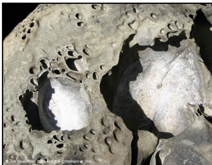
Effect of salt crystallisation on a rock
