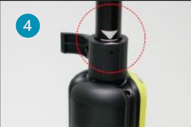
Insert antenna and match the marks
