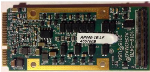
Plug-In miniPCIe with standardized Midplane I/O connector
