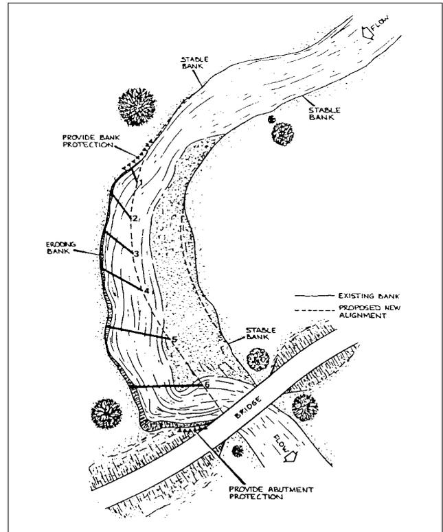
Groynes direct the main flow of water back into the main or required stream and away from eroding banks. Fences are permeable and slow water between the groynes causes sediment to deposit, which in time, establishes with vegetation and stabilises the area. However, care must be taken not to narrow the stream channel locally.
