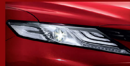
Bi-beam LED Headlamps with Follow-me-home Function & Daytime Running Lights
