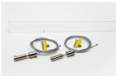
-Name: R25 - "—" type hanging mounting with PC profile -Model: R25-IA04 -Attachment: Transparent PC mounting profile, Kit of hanging rope, Screws Note: Using Transparent PC mounting profile will cause the neon body to compress and stretch, resulting in a dark area at the tail!
