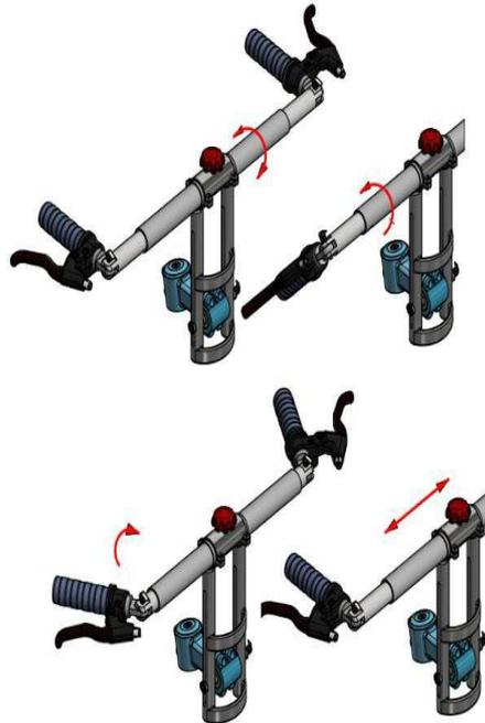
Figure 4-4 Schematic diagram of bicycle handle rotation and left and right extension
