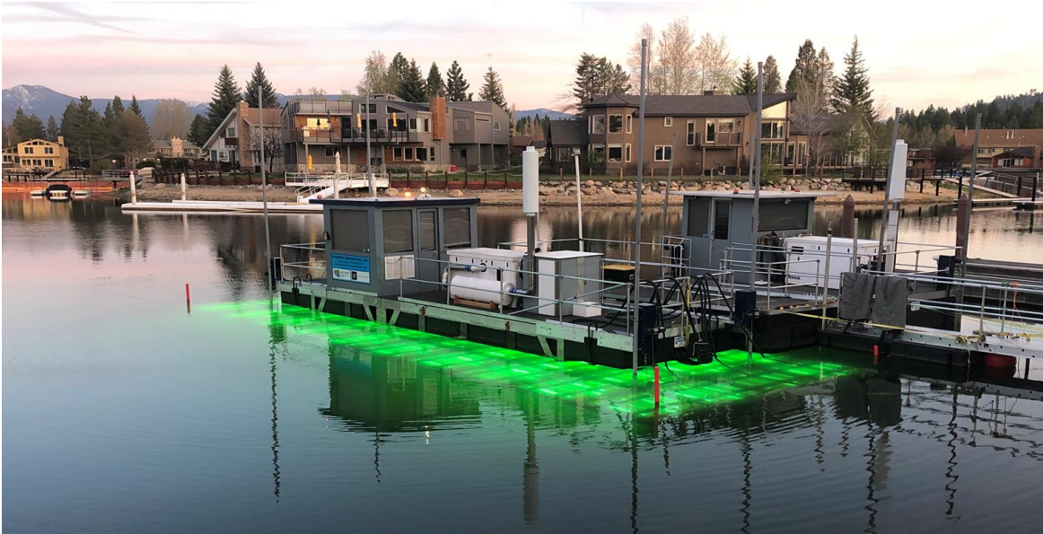
Image E - UV treatment vessel during operational testing (UV lights on).
