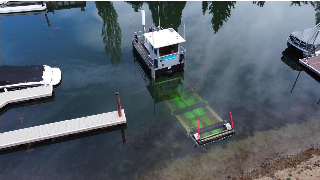
Image D - Cantilever 8ft x 40ft treatment vessel treating nearshore.
