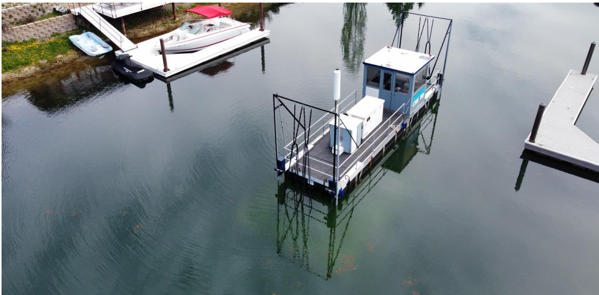
Image B - 16ft x 40ft treatment vessel treating from dock to dock at Tahoe Keys.
