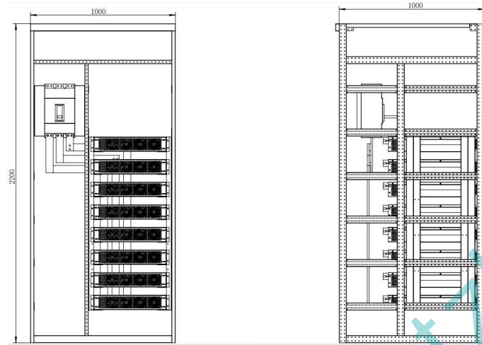
Figure 5.4: 1000k Cabinet Installation Diagram
