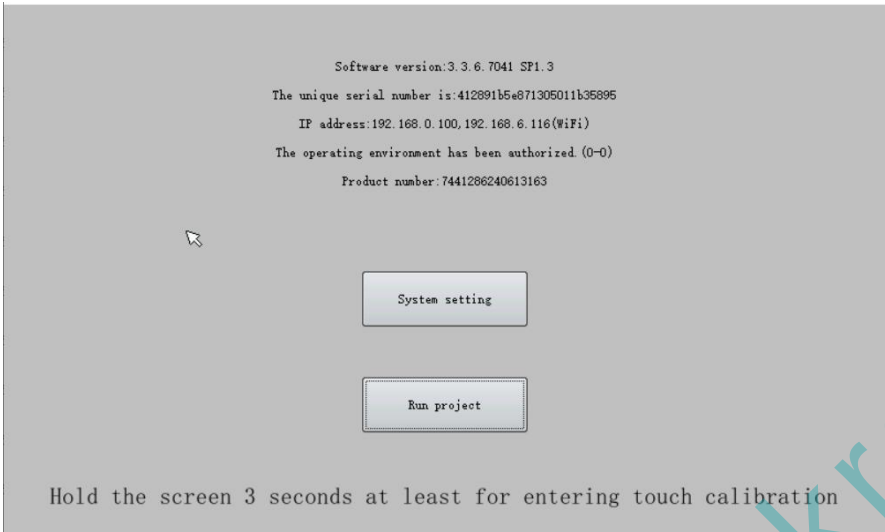
Figure 7.24: System Configuration Interface
