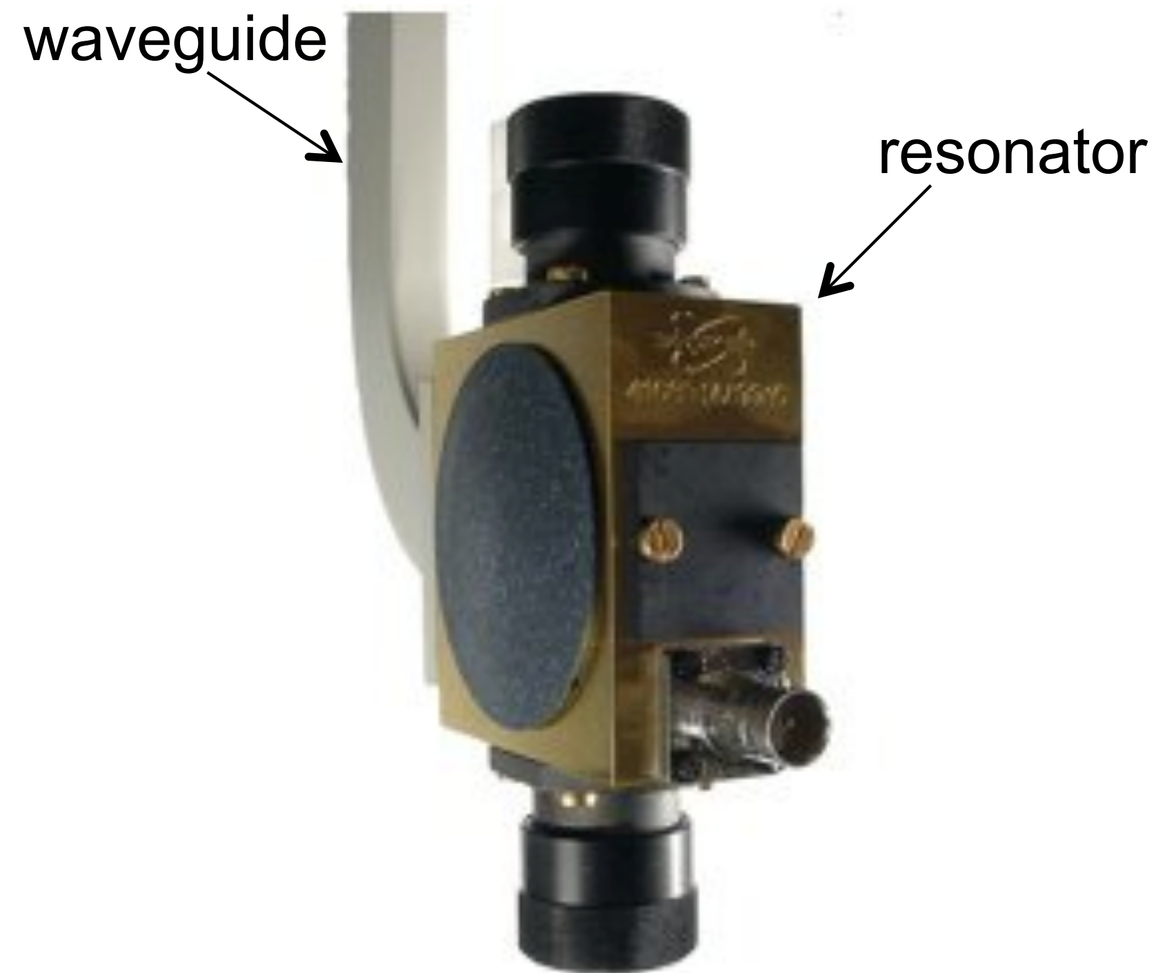
Image: Bruker ER 4103TM cylindrical mode resonator http://www.bruker.com/typo3temp/pics/e_75d2de1d39.jpg
