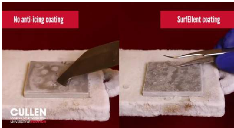
On the left, tough-to-break ice builds up on an untreated surface. On the right, SurfEllent application reduces ice accumulation and allows whatever remains to be easily removed.
