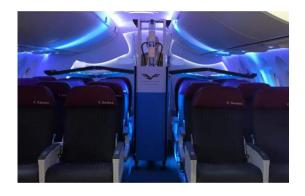
Figure 1 Fully deployed, the GermFalcon germicidal apparatus can eliminate 99.9% of viruses and bacteria on aircraft cabin surfaces in less than three minutes.
