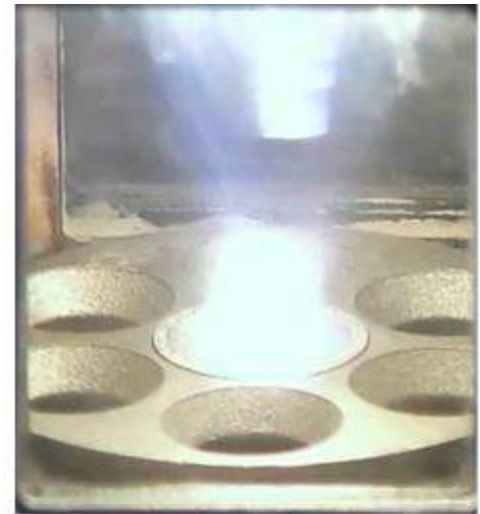
First generation plasma-assisted injector from FGC Plasma Solutions undergoing testing at NASA Glenn Research Center
