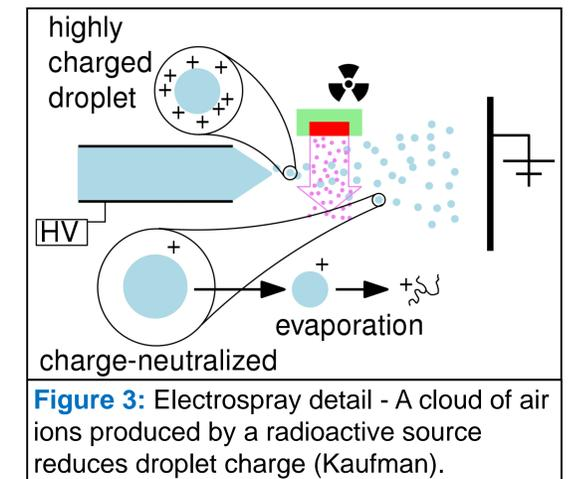
Figure 3: Electrostatic detail - A cloud of air ions produced by a radioactive source reduces droplet charge (Kaufman).
