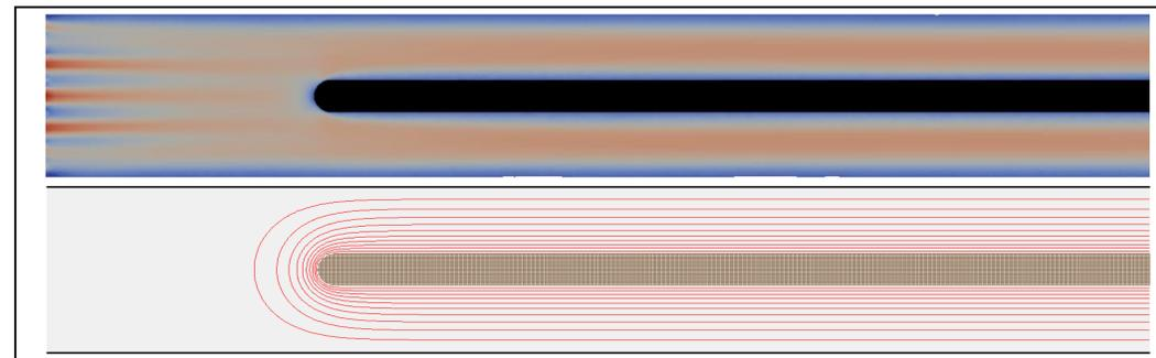
Result 1: Ion Trajectories with CFD results Compared to Constant Velocity Approximation
