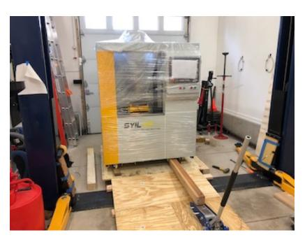
leave the machine wrapped until it is in-place, then remove the wrap. This way the outer surfaces are protected as it is moved into place.
