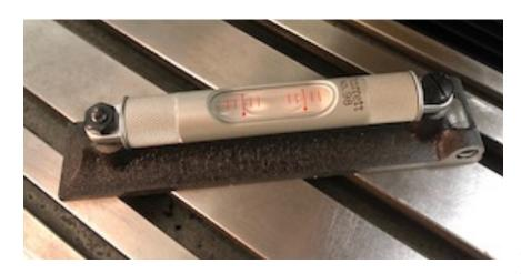
One can start with a small carpenter level, but leveling should only be completed using a machinist level, such as a Starrett No. 98 level. Perform leveling front-to-back first (along the Y axis) then side-to-side (along the X axis). Place the level along the Y axis, in the center of the table
