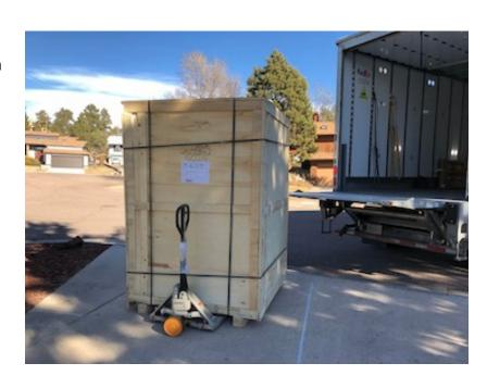
move the machine from the pallet to the floor, and finally how is it moved into the desired location. Things to consider: what additional equipment might be needed, will a forklift be needed (or other equipment) to get the machine off the pallet? Once the machine is on the floor, especially a concrete floor, it moves easily on the casters ... two people can easily move it in place on a flat concrete floor.
