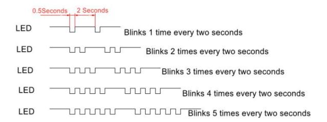
Blink 1time: Compressor stall or Compressor blockage
