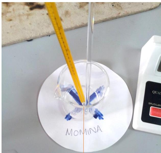
Just after the start of the reaction, the solutions are still almost clear and the blue cross is visible. Stirring rod is used to even out the concentration of reactants in the beaker, thermometer measures the rising temperature.
