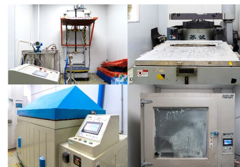
Environmental test (waterproofing/vibration/salt fog/sand dust)
