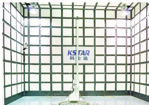
3m anechoic chamber
