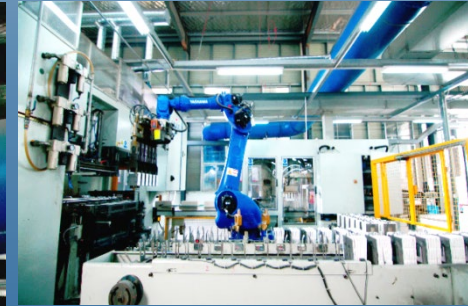
Fully automatic cast welding
