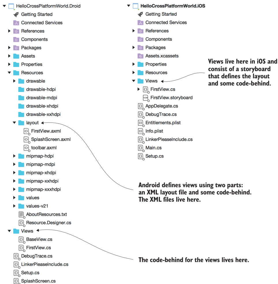
Figure 2.16 The structure of the iOS and Android app projects
