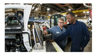
The Diesel Truck/Heavy Equipment program utilizes Caterpiller and Cummins, for engine troubleshooting, diagnostic repair, and engine rebuild. The diesel program also relies on Peterbilt and Kenworth for heavy duty vehicle electrical systems, air systems, brake systems, and power train systems. In addition, the faculty help students understand how to apply theory to a work situation and helping them gain the confidence to take on complex tasks and be
