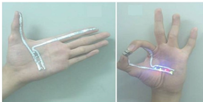
Fig. 5.4 Liquid metal as a display of skin electrons [43]. Reprinted under Creative Commons Attribution License
