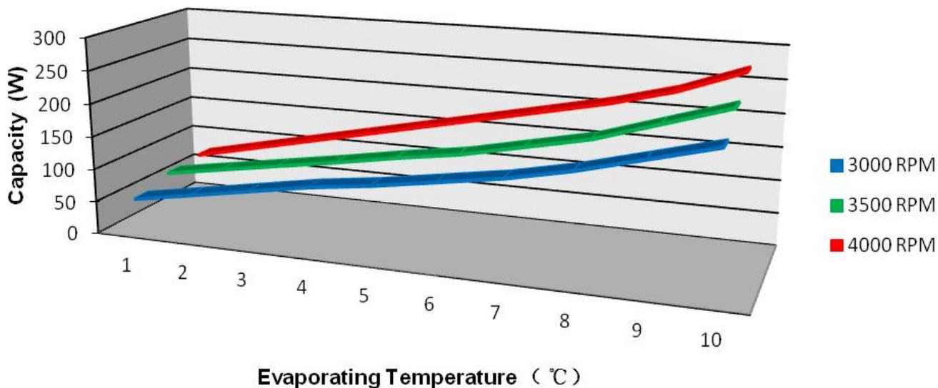
Evaporating Temperature °C      Remark: Condensation Temperature: 38°C
