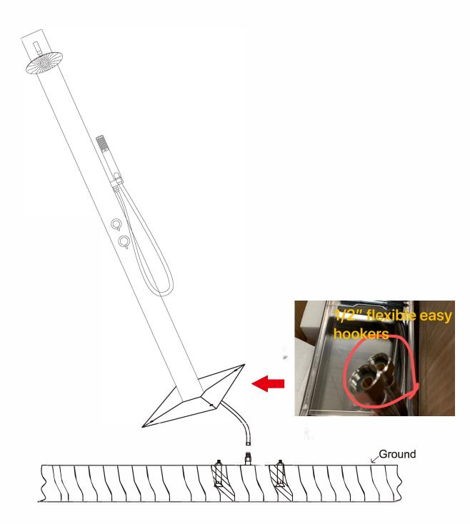
connect installed 1/2" flex water connectors to water service, level the base plate properly and ensure the placement is properly
