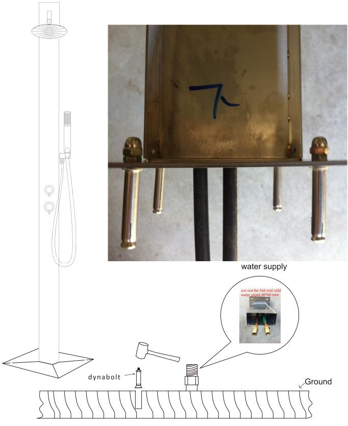
Hammer the dynabolts into the hole in the concrete 1/2" inch water pipe with male compression unions, 270mm above the ground
