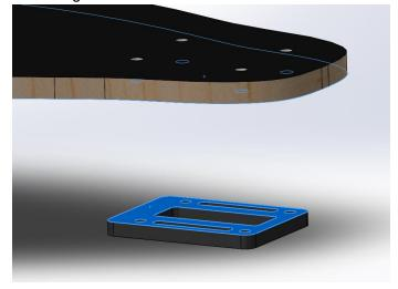
4. **Concentric mates**: Create concentric mates between the following faces of the **deck** and **baseplate**
