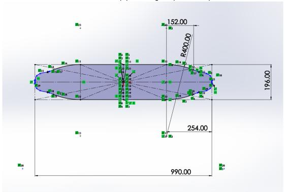
2. **Sketch 2**: Create sketch shown on right plane, connecting the ends of the sketch 1 and creating the curve of the longboard
