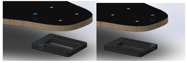
3. Tangent Mate: Create tangent mate between faces on the deck and riser
