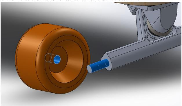
15. **Coincident mate**: Create coincident mate between the following faces on the **wheel** and **trucks**
