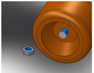
17. **Coincident mate**: Create coincident mate between the following faces on the **wheel** and **hex nut**
