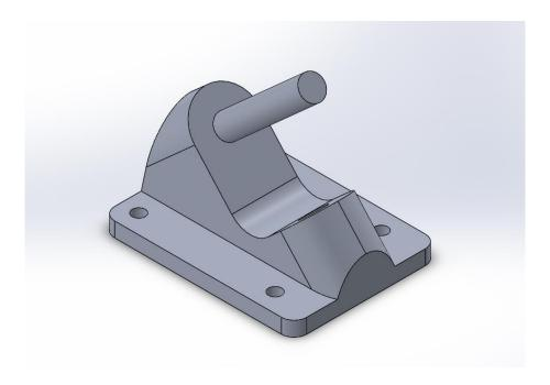
1. Boss – Extrude Base: Create sketch on top plane and extrude 5.80mm
