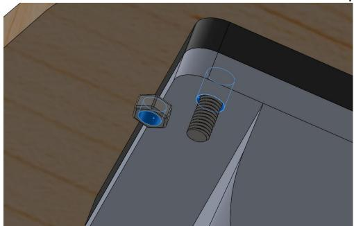
22. Coincident Mate: Create a coincident mate between the screw but and baseplate
