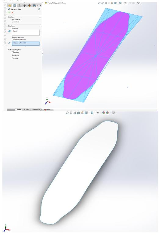
10. **Surface – Thicken 1:** Thicken surface, input 10mm.
