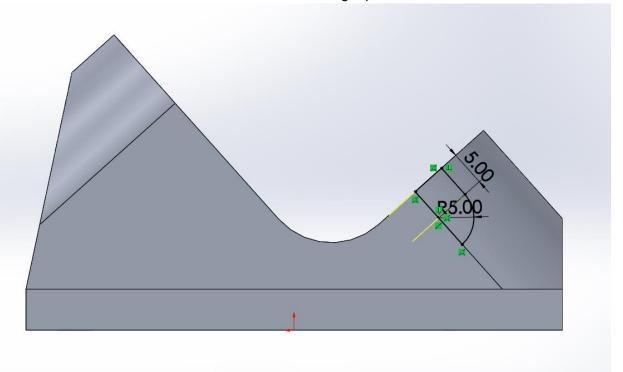
7. Boss - Extrude Shaft: Create sketch shown, concentric to fillet, and enter 45.00mm
