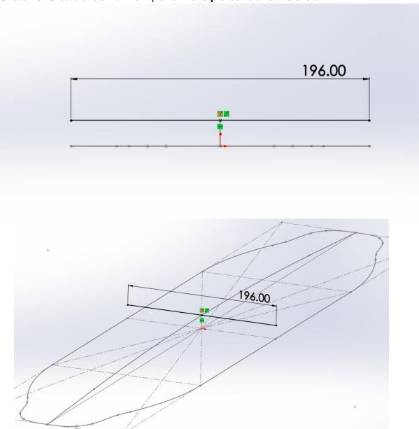
4. **Plane 1**: Create reference plane 1, parallel to front plane, coincident to furthest point in sketch 1.
