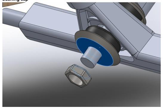
14. Concentric mate: Create concentric mate between the wheel and trucks
