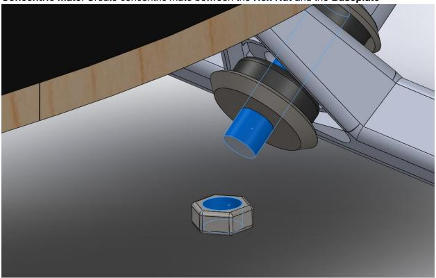
**13. Coincident mate**: Create coincident mate between following faces on the **Hex Nut** and **bushing cap**
