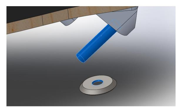
7. Coincident mate: Create coincident mate between the following faces of the bushing cap and the baseplate.
