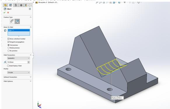
5. Fillet 2: Create a fillet selecting the four edges shown. Enter 13.00mm
