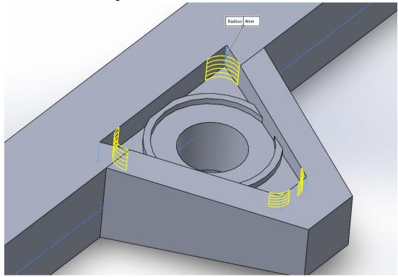
**8. Chamfer**: Select the surrounding edges of the divot and chamfer. Enter 3.00m @ 45 degrees
