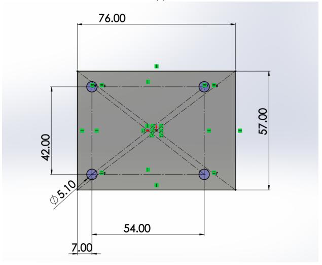
2. Boss – Extrude Plate: Create sketch on top of extrude base and extrude 60.00mm
