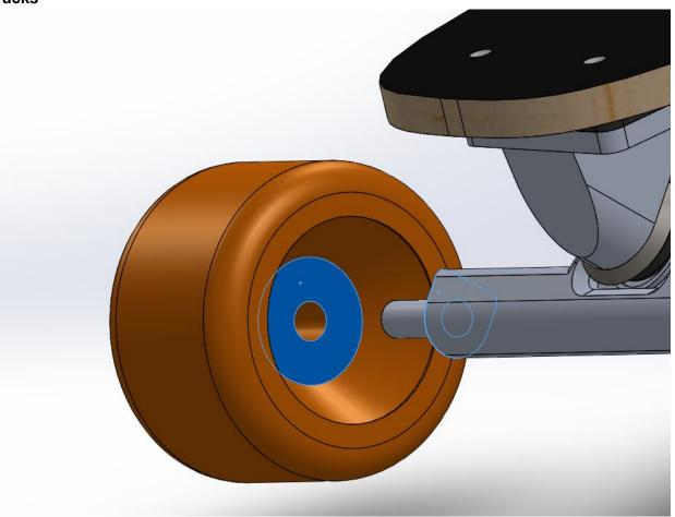
16. Concentric mate: Create concentric mate between the Hex Nut and Trucks
