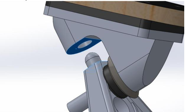
12. Concentric mate: Create concentric mate between the Hex Nut and the Baseplate
