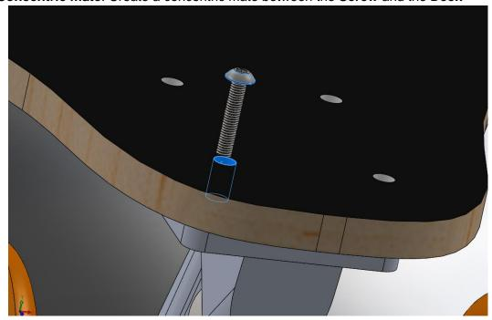
**20. Tangent Mate:** Create a tangent mate on the following faces between the **screw** and the **deck**
