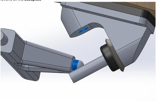
11. **Coincident mate**: Create coincident mate between the following faces on the **trucks** and the **baseplate**
