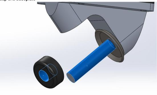
9. **Coincident mate**: Create coincident mate between the following faces on the **bushing** cap and bushing
