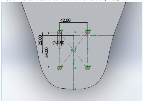
13. **Mirror – Screw Holes:** Use mirror feature to mirror the extrude cut, using the front place as the mirror plane.
