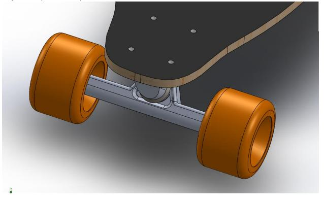
19. Concentric mate: Create a concentric mate between the Screw and the Deck
