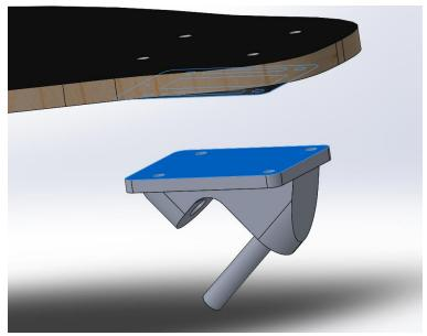
**6. Concentric mate**: Create concentric mate between the following faces of the **bushing** cap and the **baseplate**.
