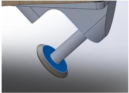
8. Concentric mate: Create concentric mate between the following faces on the bushing cap and baseplate
