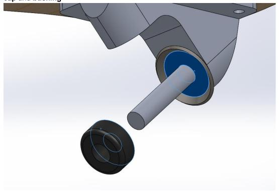
10. **Concentric mate**: Create concentric mate between the revolve on the **trucks** and the revolve on the **baseplate**
