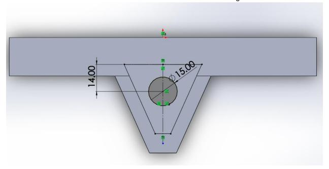
**5. Boss – Bushing Walls**: Create a circle with a diameter of 5.50mm, concentric to shaft hole, and offset circle by 1.50mm. Extrude by 1.50mm.
