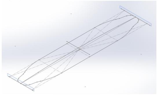
8. **Surface – Loft 1**: Create a surface loft with sketches 4, 5, and 6 for the profile and sketch 2 as the guide curve.
