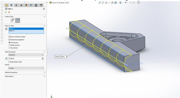
12. Fillet 3: Perform a fillet on the front nose of the trucks. Enter 3.00mm
