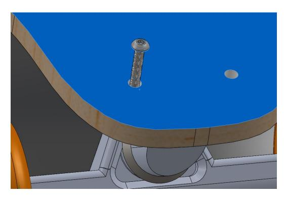
21. Concentric Mate: Create a concentric mate between the screw nut and baseplate
