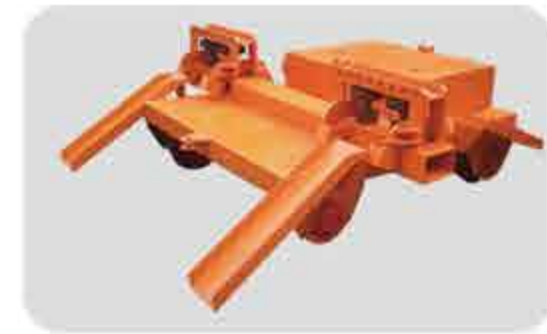
换轨车(一车) Rail replacement vehicle (No.1)
