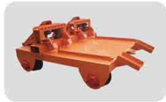
换轨车(二车) Rail replacement vehicle (No.2)
