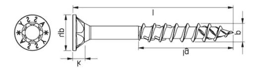
These WURTH screws combined with the RW20 bit are the best to install climbing holds to wooden panels with ease. Many climbing centres in Australia, Europe, Asia, etc. have been using these screws in recent years and there is no going back!
