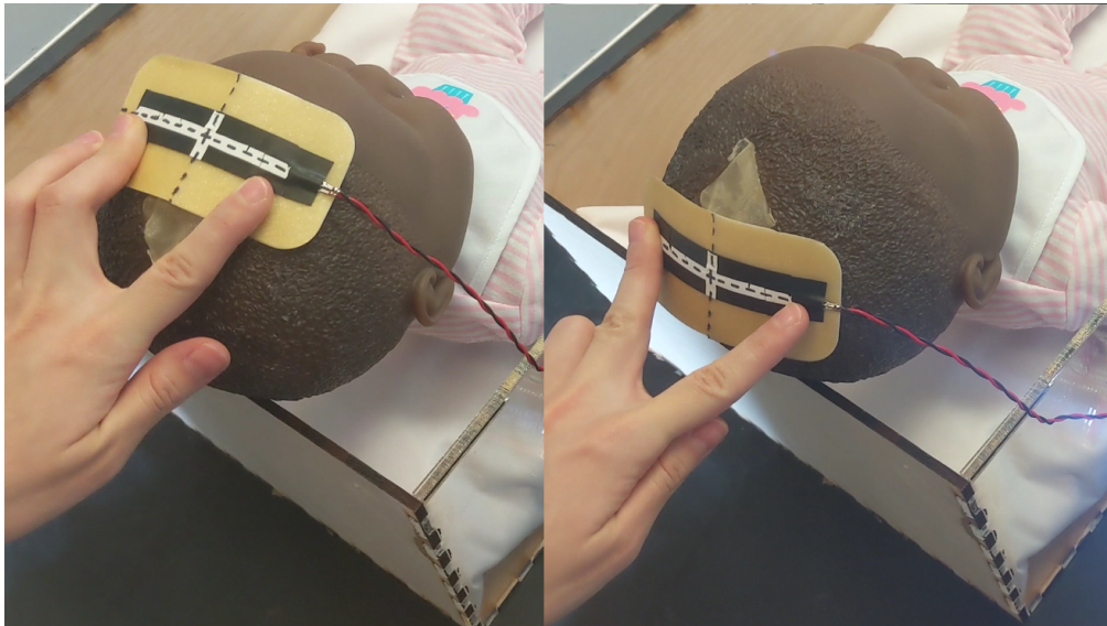
Figure 31: Calibration for Head Curvature. Left: Sensor at the Front of Fontanelle. Right: Sensor at the Back of Fontanelle.
