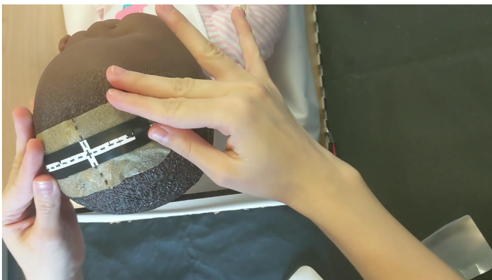
Figure 32: Attaching the sensor. Left: Matching the guide lines. Right: Patting down the adhesive.
