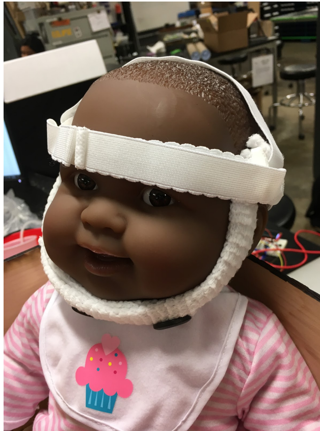
Figure 13: Attachment Method 2 - Using Straps to Secure Under the Chin and Around the Head
