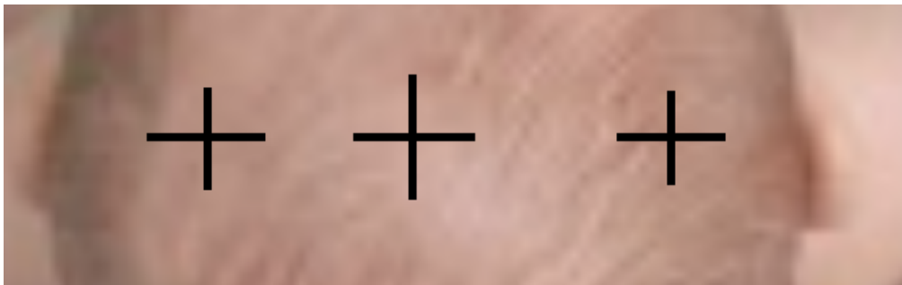
Figure 40: Locations to mark on baby head model for helmet movement testing. (Top View)
