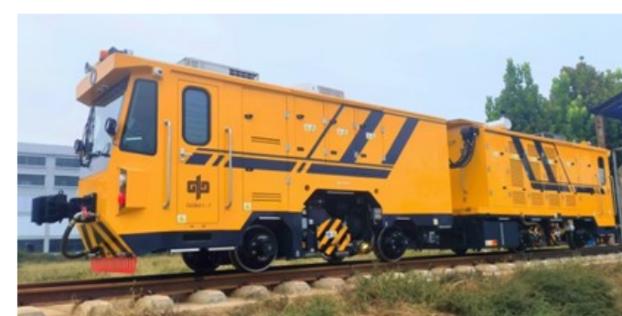
FGM500C Rail Milling Train (Zhengzhou Metro, China)
