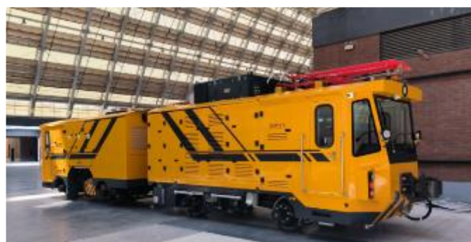
FGM500B dual-power Rail Milling Train (Guangzhou Metro, China)
