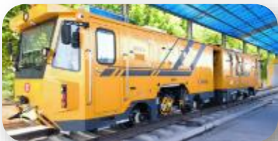
FGM500A Rail Milling Train
