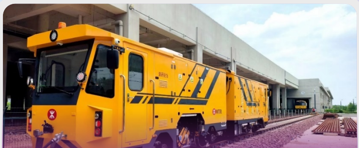
FGM500A Rail Milling Train
