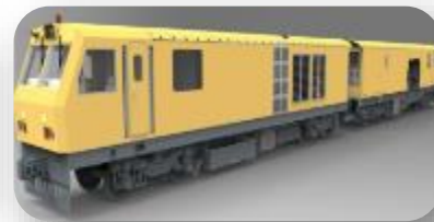
High-speed rail milling machine
