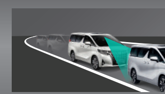
Lane Tracing Assist (LTA)* Keeps the vehicle centered either by detecting the lane or the preceding vehicle.
