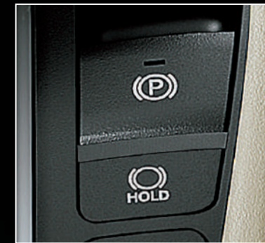
ELECTRIC PARKING BRAKE (EPB) WITH BRAKE HOLD Keeps the vehicle stationary on flat roads with a simple button. Automatically releases during acceleration.
