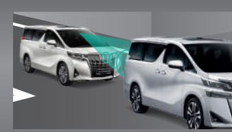
Pre-collision System (PCS)* Avoids or mitigates frontal collisions by alerting the driver and automatically applying the brakes when there is a risk of collision.
