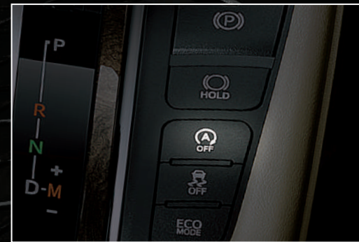
AUTO START-STOP SYSTEM Automatically stops the engine when vehicle is stationary for enhanced fuel economy. As soon as the brake pedal is released, the engine restarts immediately.
