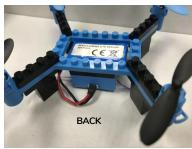
9) Secure the battery by placing four 1x5 Lego pieces on top, attaching/connecting the ends of the Lego pieces to the drone. These should be placed in the middle part of the center.
