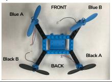
7) Add a 1x4 black Lego piece to the bottom of each propeller. Then stack four 1x2 Lego pieces on top of each other until you have four stacks. Attach one stack on each leg.
