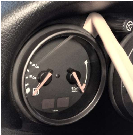
Figure 1 Use plastic pry tools to loosen gauge.
