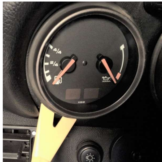
Figure 1 Use plastic pry tools to loosen gauge.
