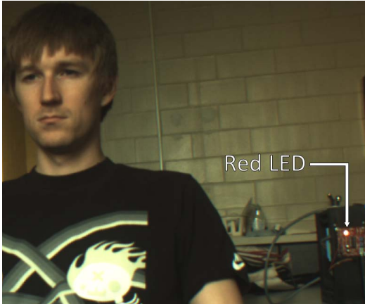
Fig. 2. Example frame from our recorded data set. Ambient light was used to illuminate the face while ground truth data was acquired from a red LED, which turned on with each heart beat, placed behind the subject.
