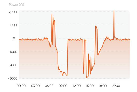
Inverter disconnecting due to network overvoltage in Gridsight
