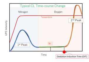
The graph on the left shows typical CL behaviour during heating measurement. As the sample is heated, the peroxide decomposes, and CL from the excited carbonyl increases, resulting in a peak (the first peak). This corresponds to the amount of peroxide at that point.
