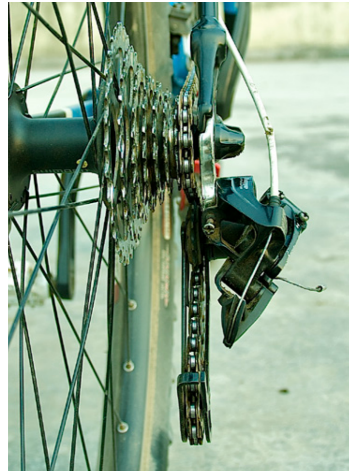
TIGHTEN THE SCREW TO MOVE THE DERAILLEUR INWARDS, LOOSEN TO MOVE IT OUTWARDS
