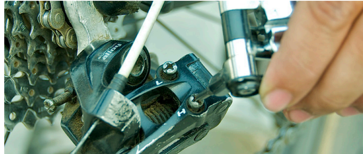
TIGHTEN THE SCREW TO MOVE THE DERAILLEUR INWARDS, LOOSEN TO MOVE IT OUTWARDS
