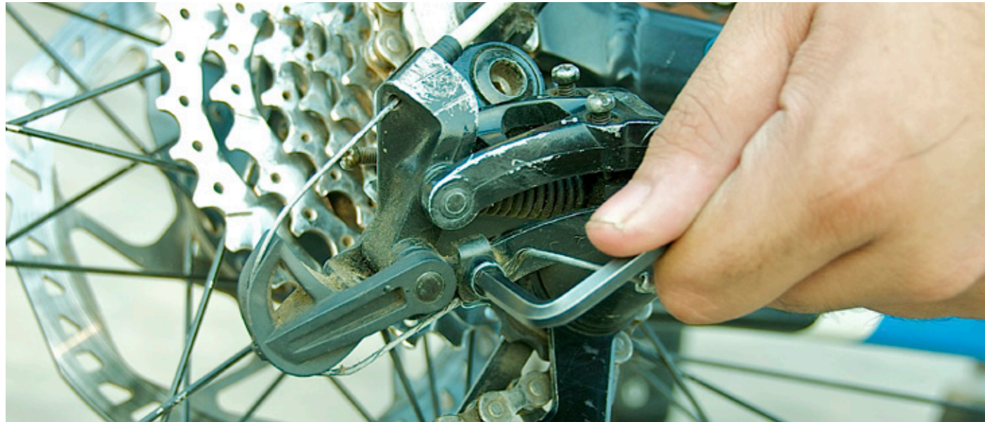
LOOSEN THE BOLT THAT HOLDS DOWN THE CABLE, SO THE DERAILLEUR IS COMPLETELY FREE
