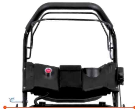
E-Start Panel with Battery Slot
