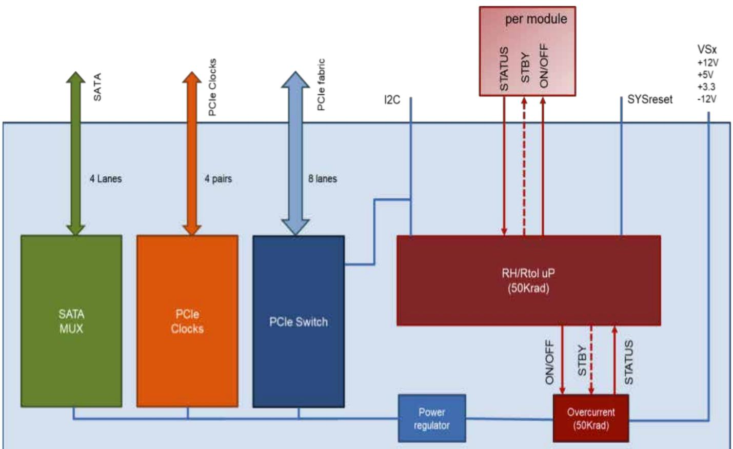
Figure 4 — Block diagram of System Controller Module.
